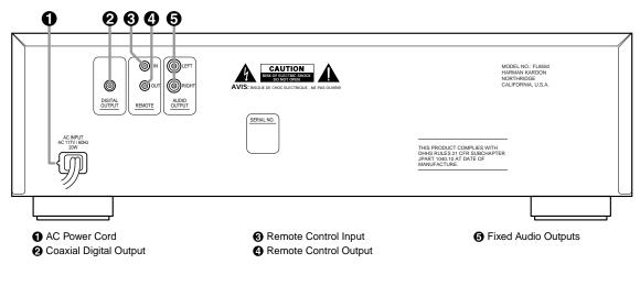
**()** AC Power Cord: Connect this plug to an AC outlet. If the outlet is switch controlled, make certain that the switch is in the ON position.
